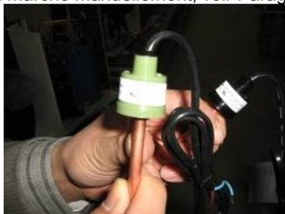
Figure 27: Pressostat de pression maximale.
